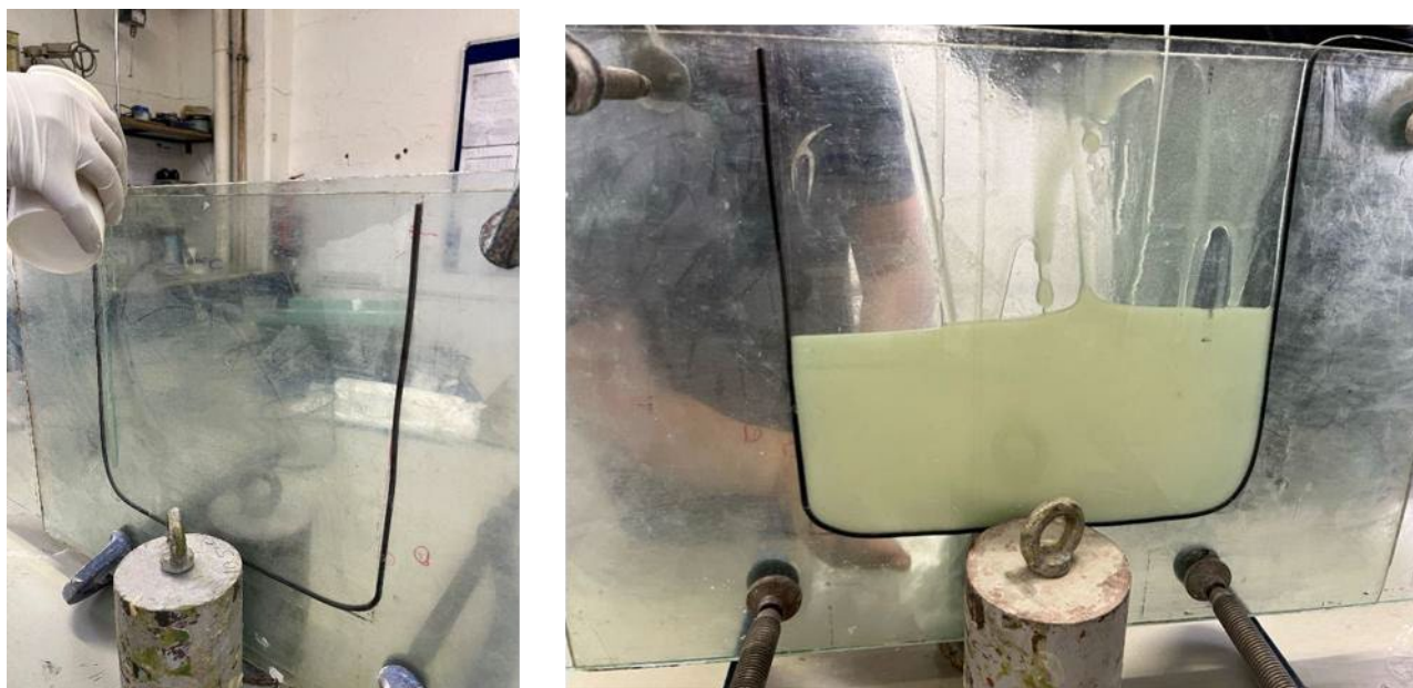
Figure 3.7: Conventional casting of epoxy resins
