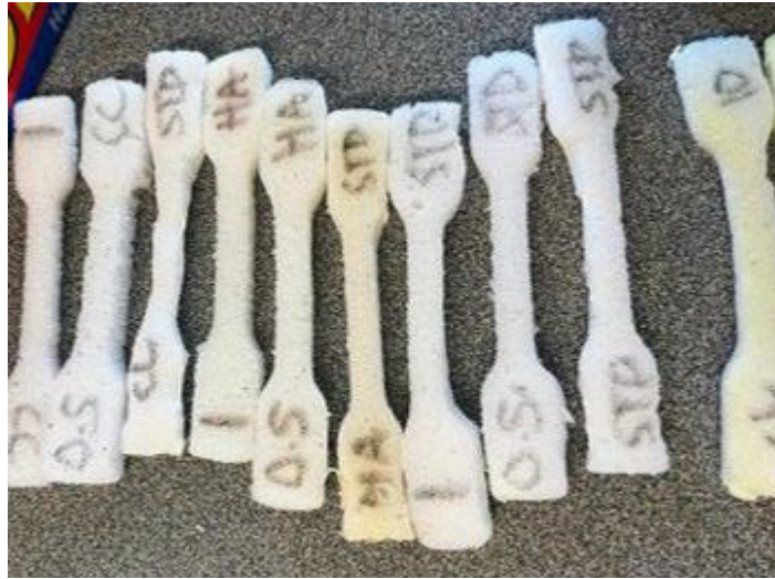
Figure 3.9: PUF tensile specimens
