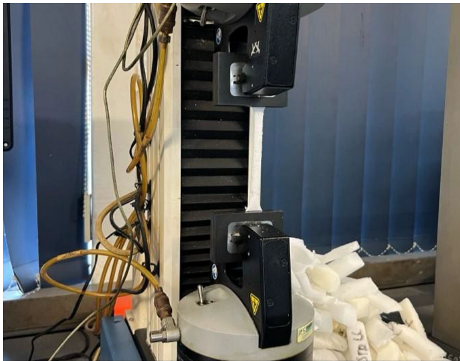
Figure 3.10: Testing tensile strength of PUF
