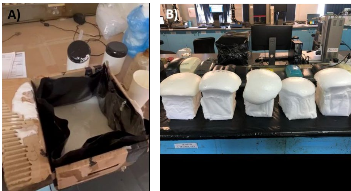
Figure 3.6: PUF (A) creaming and rising; (B) formed PUF foam
