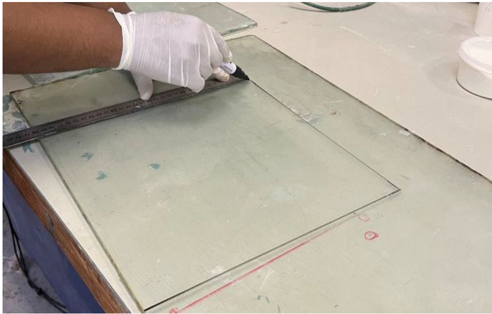
Figure 3.8: Machining out epoxy specimens
