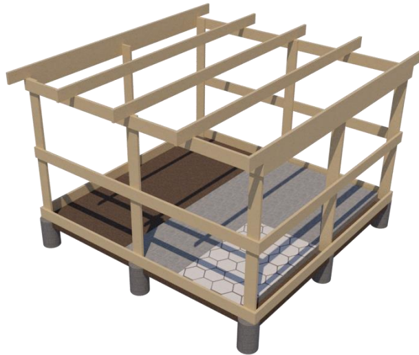
Figure 49. Concrete screed laid on hardened earth, finished with a PVC and/or vinyl flooring in QRWIS. Source:
