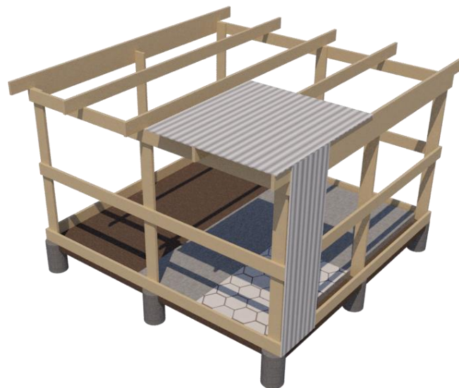
Figure 48. Corrugated iron sheet cladding in QRWIS. Source: Author
