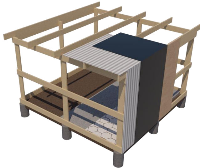
Figure 50. PVC membrane as additional waterproofing and air tightening solution in QRWIS. Source: Author
