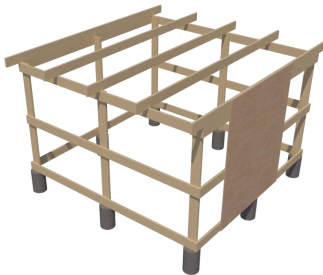
Figure 47. Plywood cladding in QRWIS. Source: Author
