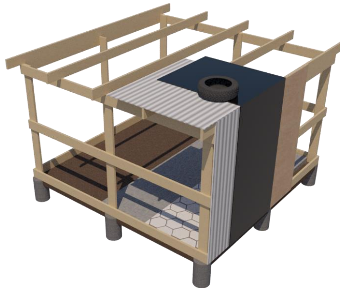
Figure 51. Use of tyres as structural element against wind loads in QRWIS. Source: Author
