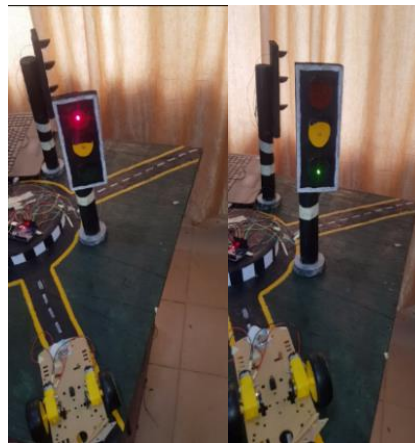
Figure 6. Traffic light signaling to the ambulance approaching
