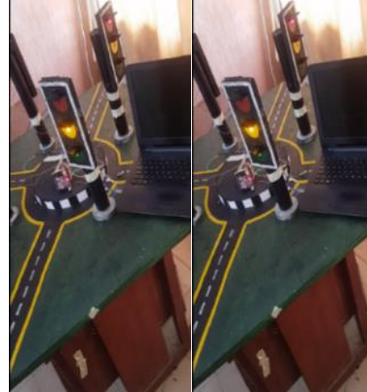
Figure 5. The traffic light board shows a yellow light on the first lane
