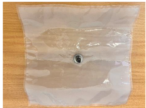
Figure 3-8: A) Gas analyser for biogas characterization and B) Tedlar bag for biogas collection
