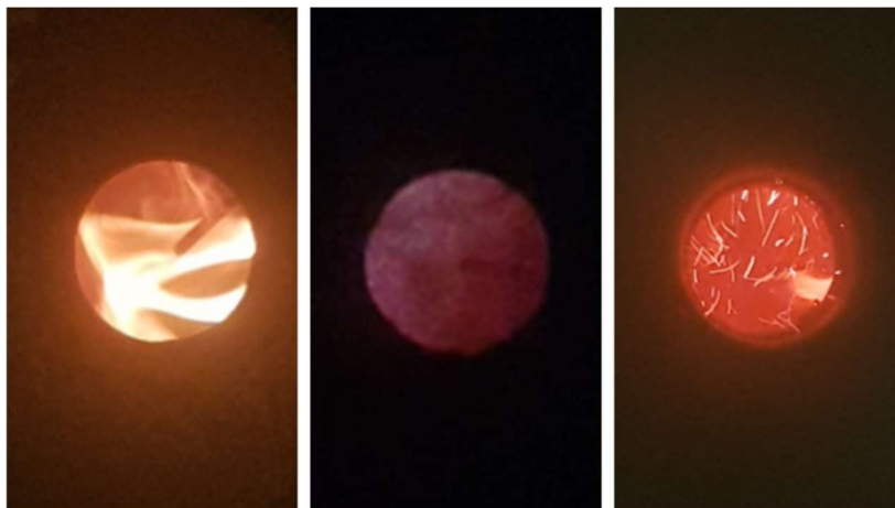
Figure 4: Left: Combustion of LPG below autoignition temperatures Centre: Combustion of LPG above autoignition temperatures Right: Combustion of the biochar during normal operation
