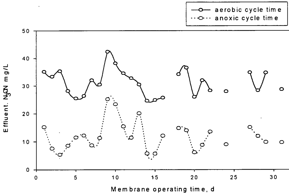
Figure 5.21 - Effluent nitrate concentration during intermittent aeration
