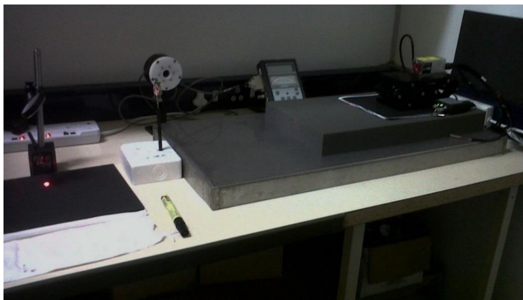
Figure 2.1 Set-up of the red light diode laser system at a wavelength of 661 nm with a spot size of 1 cm (diameter) used to deliver light doses of 2.5 J/cm 2 , 4.5 J/cm 2 and 8.5 J/cm 2 to monolayer of cells seeded in 24-well plates.
