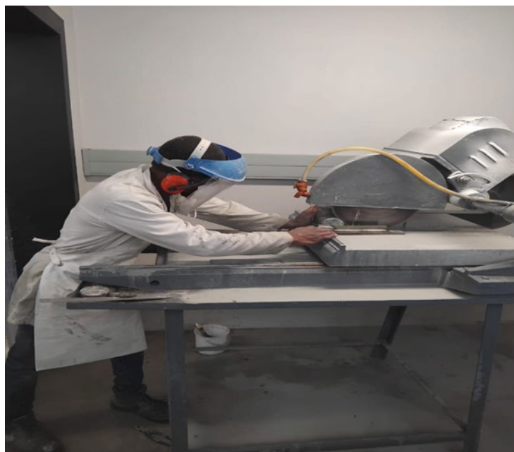
Figure 3.19: Cutting of concrete samples (Photo by Peace Adedeji, taken at WITS durability laboratory, 2024)
