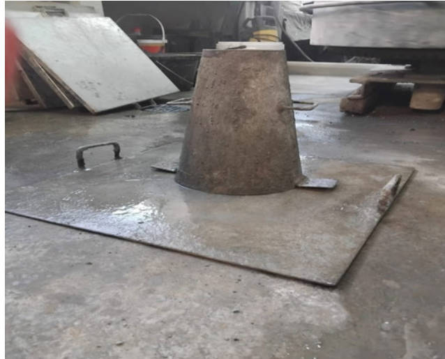
Figure 3.13: Slump test apparatus (Photo by Peace Adedeji, taken at WITS concrete laboratory, 2024)
