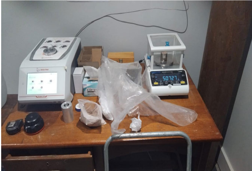
Figure 3.11: Anton Paar ultrapyc 3000 gas pycnometer density analyzer (Photo by Peace Adedeji, taken at WITS Geotechnic laboratory, 2024)
