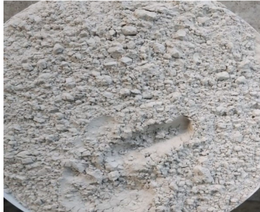
Figure 3.3: Image of GGBS obtained from Afrisam (Photo by Peace Adedeji, taken at WITS concrete laboratory, 2024)
