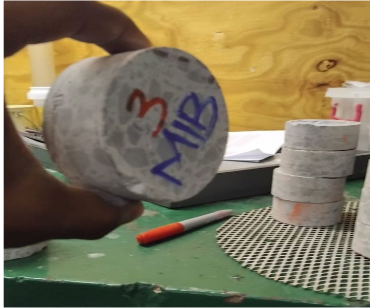
Figure 3.20: Typical disc for durability test (Photo by Peace Adedeji, taken at WITS durability laboratory, 2024)
