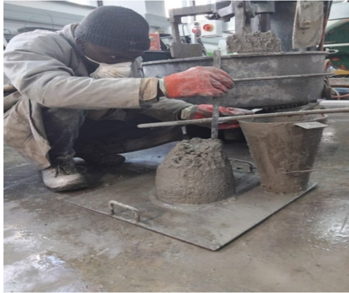
Figure 3.14: Concrete slump measurement (Photo by Peace Adedeji, taken at WITS concrete laboratory, 2024)
