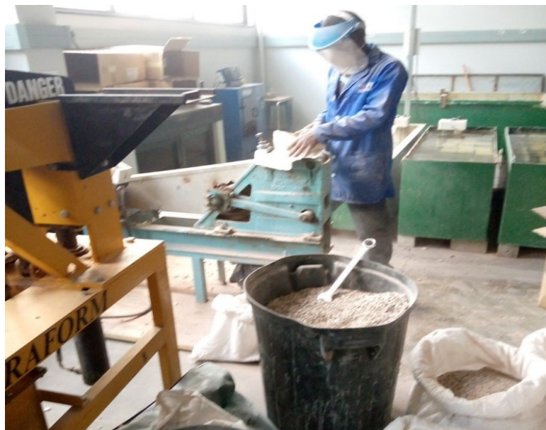
Figure 3.6: Crushing of ceramic wastes with a jar crusher (Photo by Peace Adedeji, taken at WITS concrete laboratory, 2024)
