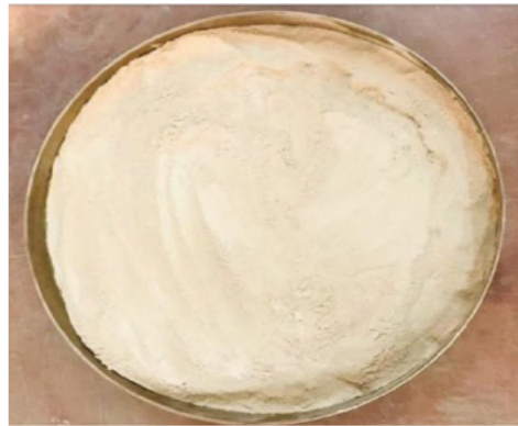
Figure 2.2: CWP obtained from final cutting and polishing stages of ceramic production (Attaelmanan, Elhaj Mahgoub Kambal & Mansour 2021)
