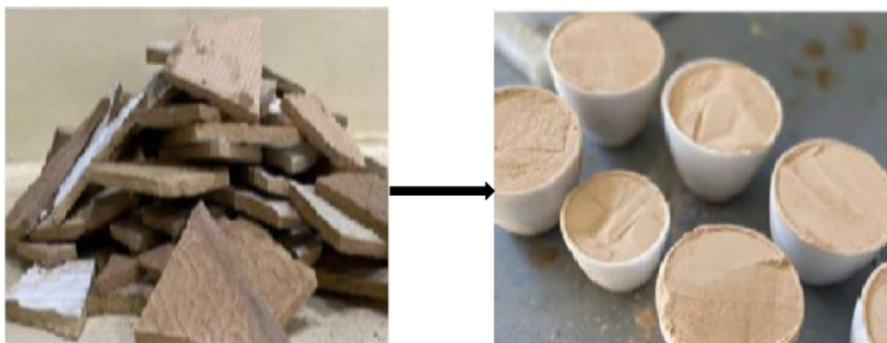
Figure 2.3: CWP obtained by crushing and milling ceramic tiles into powder (Taher, Abed & Hashim 2023)
