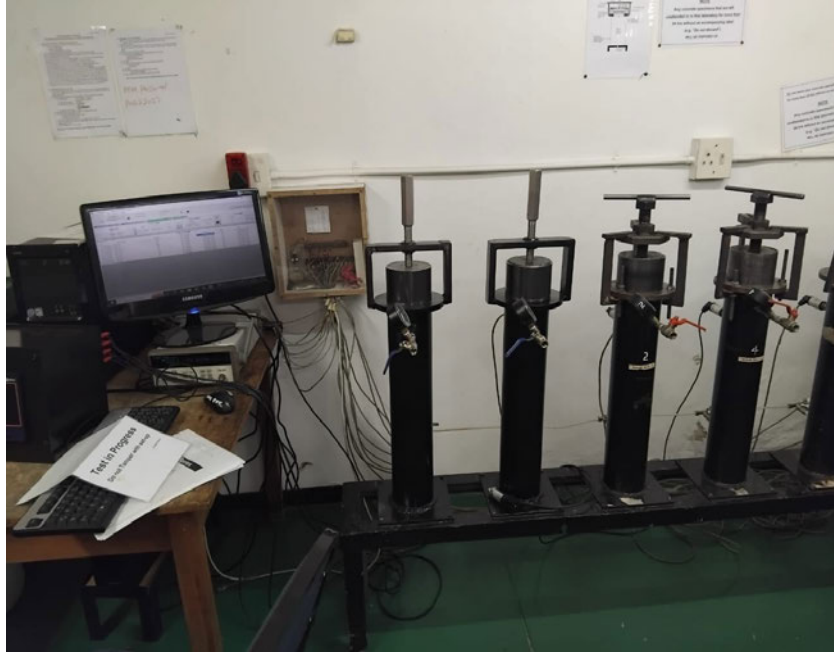
Figure 3.21: Oxygen permeability cell setup (Photo by Peace Adedeji, taken at WITS durability laboratory, 2024)
