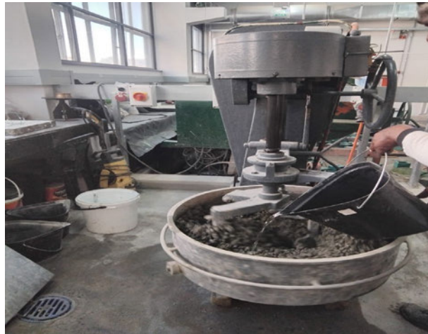
Figure 3.12: Concrete mixing (Photo by Peace Adedeji, taken at WITS concrete laboratory, 2024)
