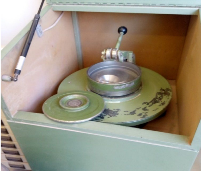
Figure 3.7: Laboratory pulveriser used to milled ceramic wastes into powder (Photo by Peace Adedeji, taken at WITS Geotechnic laboratory, 2024)
