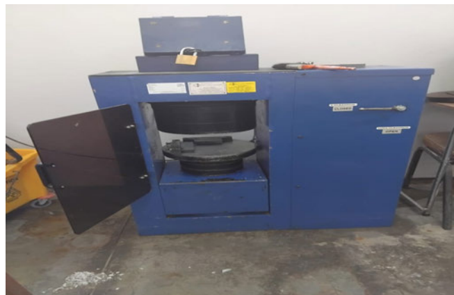
Figure 3.17: Compressive strength testing setup (Photo by Peace Adedeji, taken at WITS concrete laboratory, 2024)
