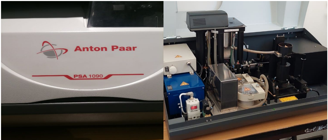
Figure 3.10: Anton Paar particle size analyser (PSA 1090) (Photo by Peace Adedeji, taken at WITS concrete lab, 2024)
