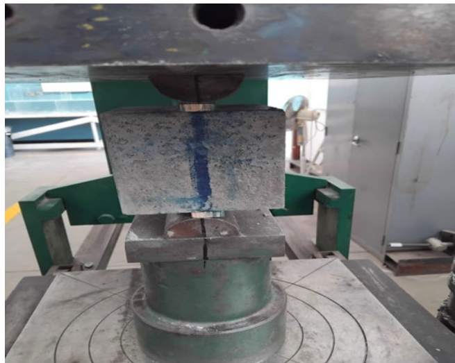
Figure 3.18: Splitting tensile strength test setup (Photo by Peace Adedeji, taken at WITS structures laboratory, 2024)
