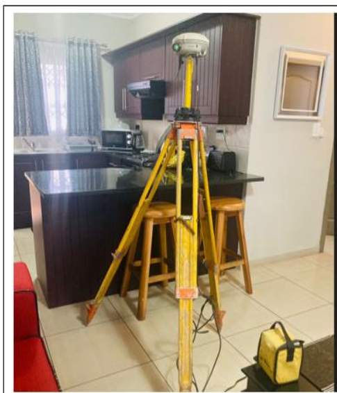
(b): Flat surface with maximum signal obstruction (GPS+Galileo signals), combined detection of the signal (Multiconstellation GNSS receiver) for indoor application
