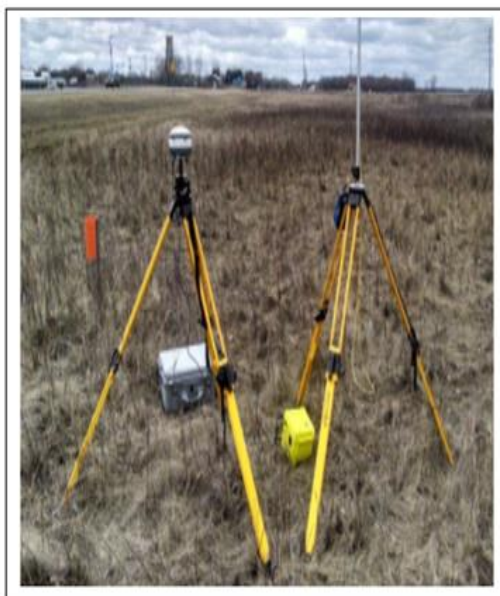
Figure 4 (a): Flat surface with no signal obstruction GPS receiver, only capable of processing GPS signals
