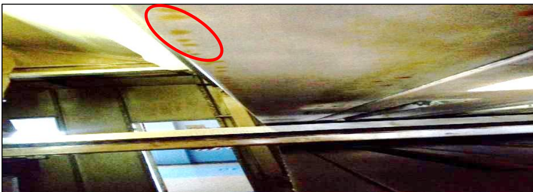
Figure 4.6: Photo illustrating oil droplets that result in product defect
