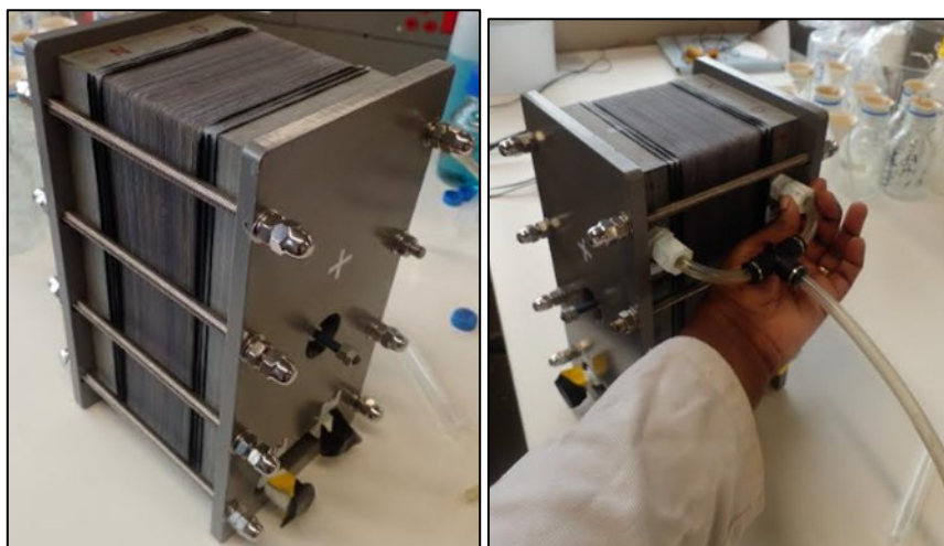
Figure 4- 2 : Assembled RED stacks with (right) and without (left) connection of rinse solution lines.
