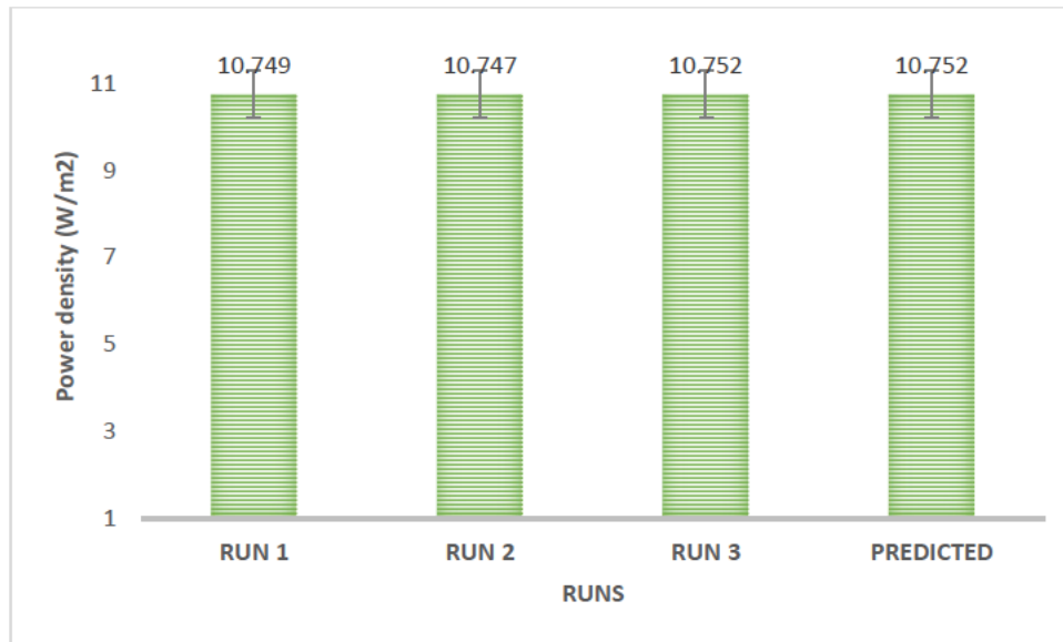
Figure 5-13: Comparing the RSM predicted response value to the experimented response of power density at temp 40°C, flow rate of 896mL/min, and high concentration of 1.93 mol/L NaCl.
