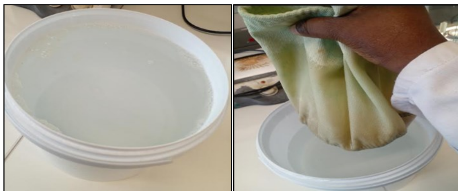
Figure 4- 10: Dirt-synthesised wastewater (left) and filtered wastewater (right).
