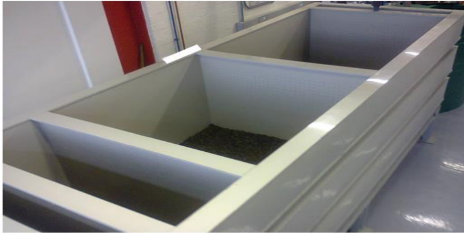
Figure 3-1: The configuration of the three compartment HRF equipment set up (Mtsweni, 2016).
