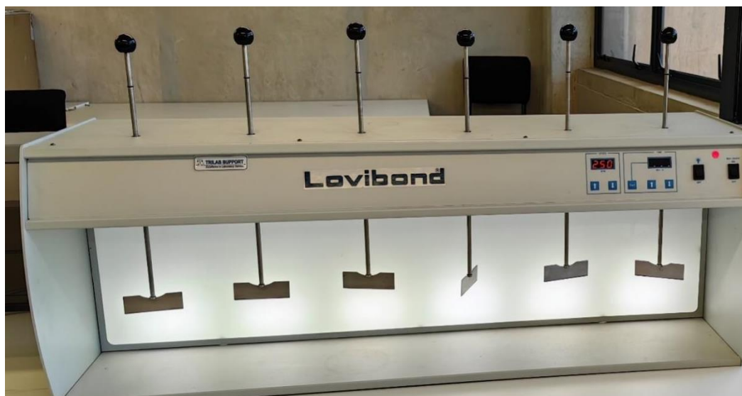
Figure 3- 3. Jar test instrument set up for chitosan experiments.
