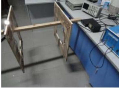
18: Figure 2.18: Proposed four-coil WPT system (Huang et al., 2014)
