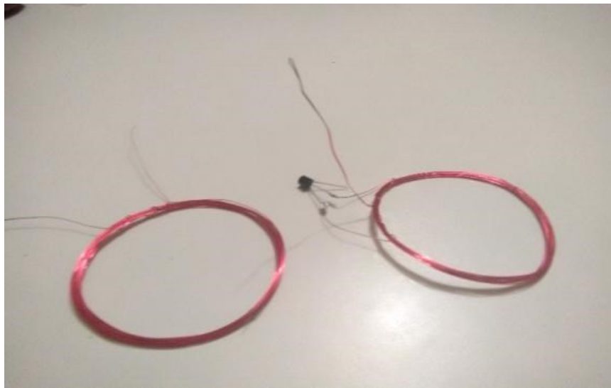
85: Figure 6.1: Photograph of the transmitting (with transistor) coil and receiving coil
