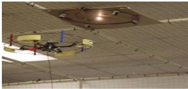
9: Figure 2.9: NIMBUS Lab's quadrotor uses strongly coupled magnetic resonance (Szondy, 2012)
