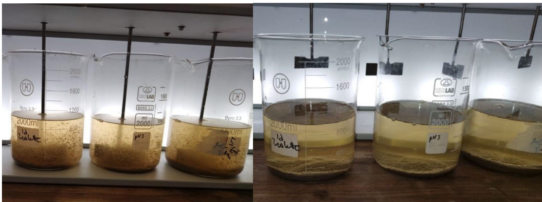
Figure 6-6: Jar tester with (a) Samples during coagulation process (b) Sample after settling.
