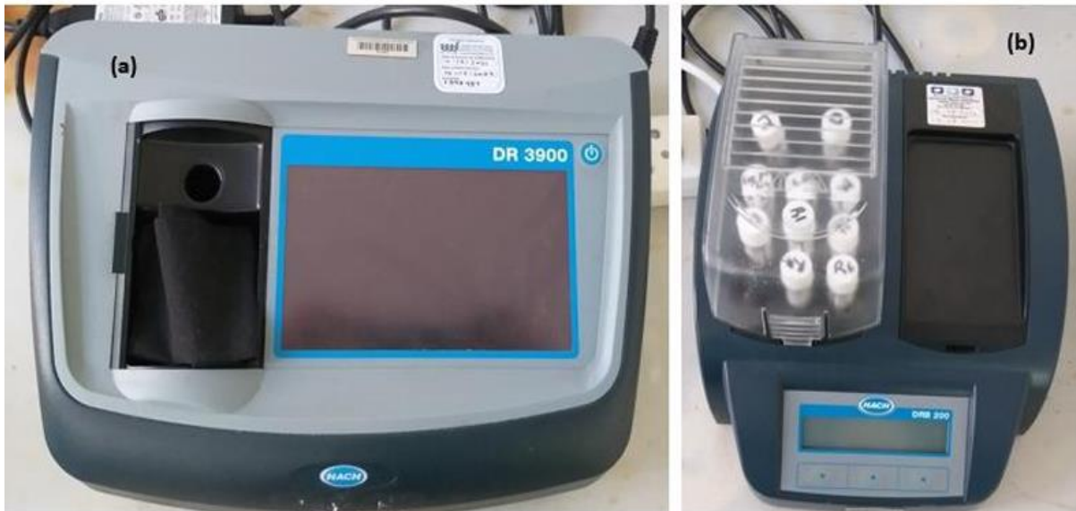
Figure 6-1: (a) HACH spectrophotometer used for contaminant analysis (DR3900), and (b) COD digester
