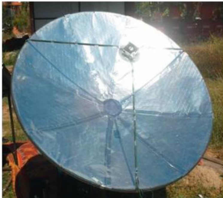
Figure 2.11: The solar parabolic concentrator coupled with the TEM [68]
