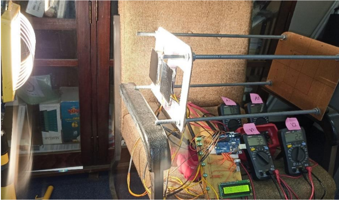
Figure 3.15: A picture of the TEG system with black coated roof sheets in closed circuit position during experiments at 600 mm
