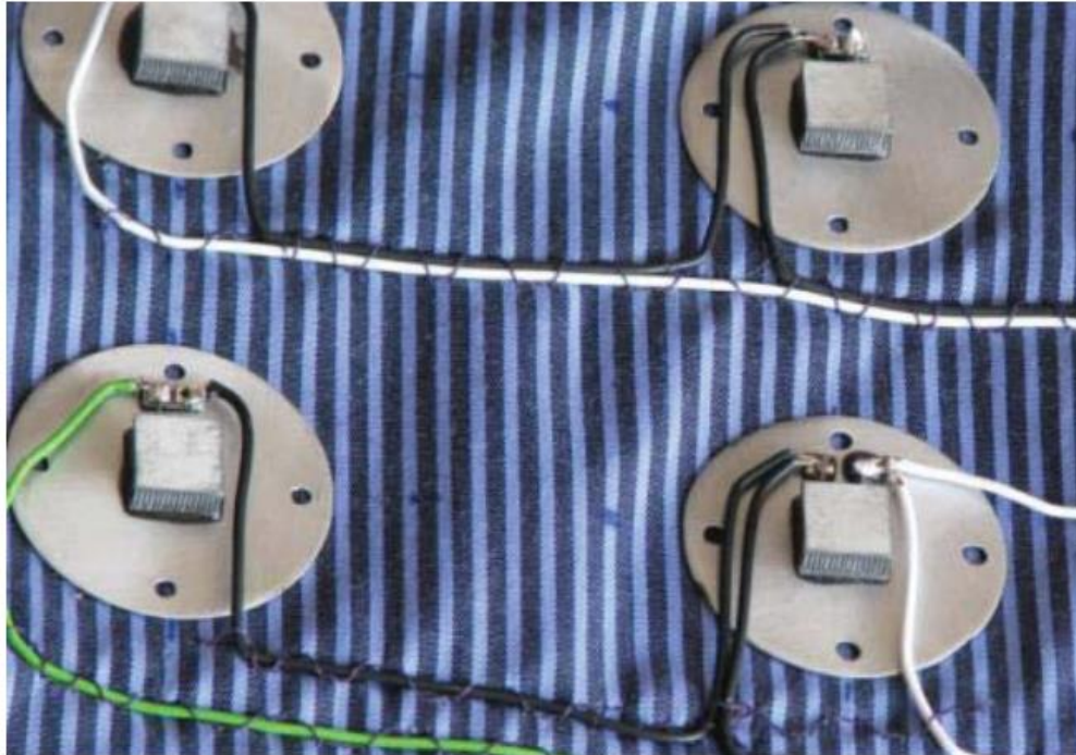
Figure 2.44: TEG integrated textile with four thermopiles assembly [109]
