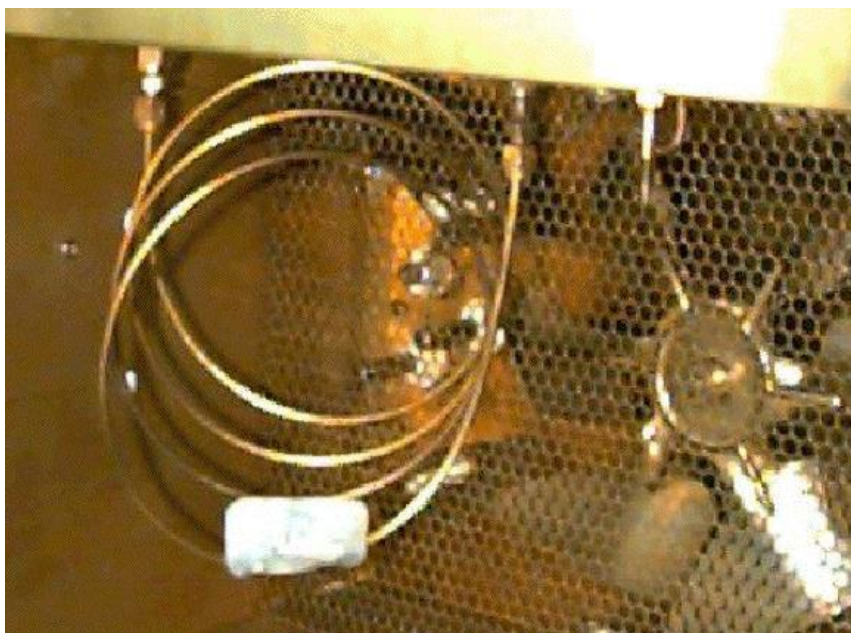
Figure 4.3.4 A diagram showing a packed column inserted into a gas liquid chromatography oven.
