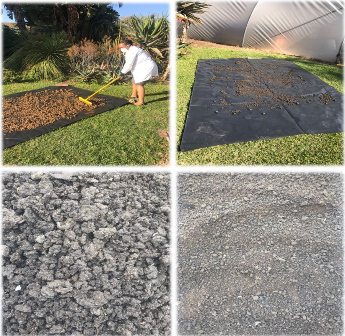
Figure 3.1 Showing the drying process and the reduction of particle size of sewage sludge after grinding
