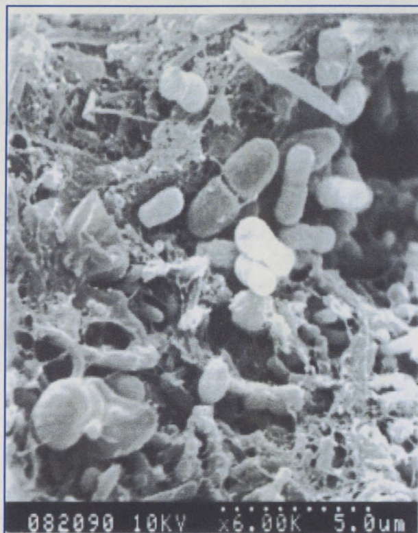
FIGURE 4.53 Environmental scanning electron micrographs of a microbial floc from the oil effluent treatment process pre-treated with a non-polar solvent. Scale bars and magnification is reflected at the bottom of the micrograph.
