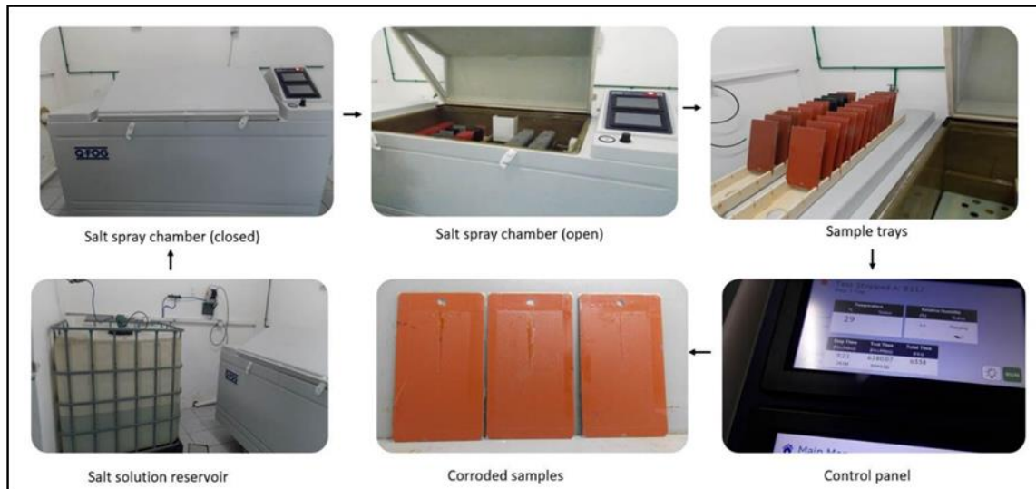
Figure 3:3. Illustration of a salt spray chamber adhering to test method ASTM B117.
