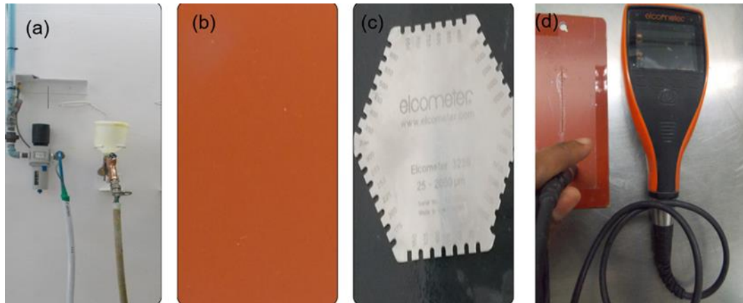
Figure 4:5. Salt spray panel preparation, (a) conventional air assisted spray gun; (b) nano-coated material; (c) Dry film gauge and (d) WFT Guage.
