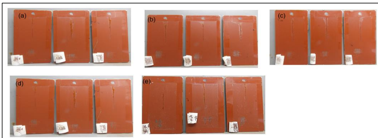
Figure 5:12. Cross-cut adhesion test results on the ss exposure of WBA composites on MS (a) WBA- Zn_3(PO_4)_2 ; (b) WBA-GO; (c) WBA-PVP; (d) WBA-GO/PVP and (e) WBA- Zn_3(PO_4)_2 / PVP.
