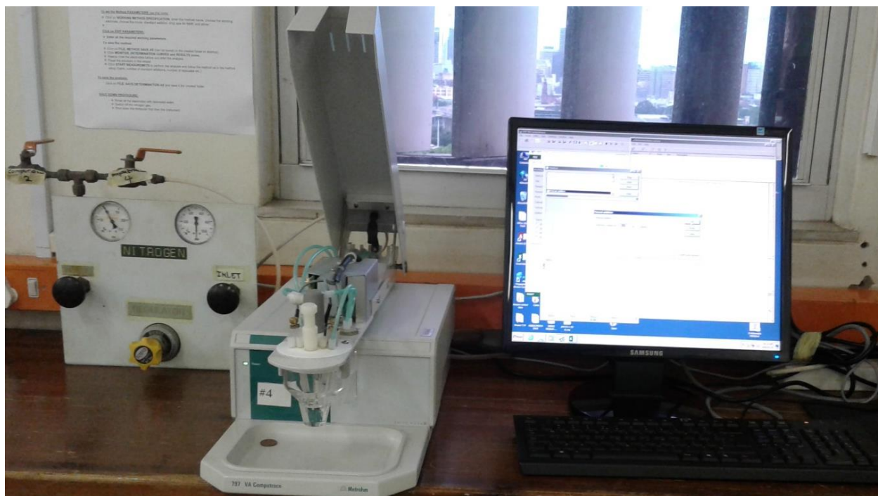
Figure 3.1: A pictorial representation of voltammetry instrumentation
