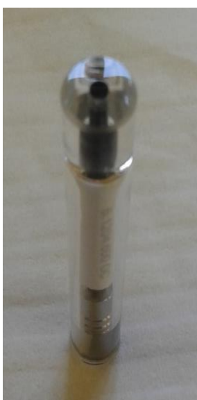
Figure 3.2: Unmodified glassy carbon electrode representation
