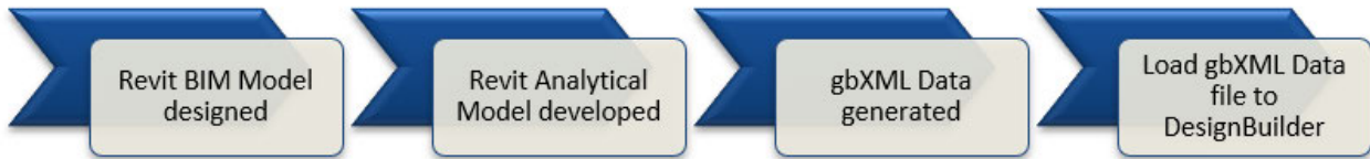
Figure 5.4: Schematic procedure of converting Revit data to DesignBuilder
