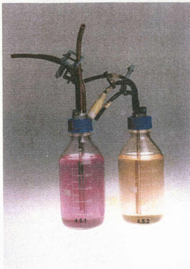
Figure 4.5 Modified Rogers bottle for the preparation of pre-reduced media
