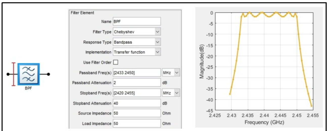
Figure 3.21: BPF simulation setup and frequency responses, 2.4 GHz
