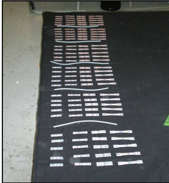
Figure 3: 120 specimens from top to bottom, the six groups (G0 to G25) and from left to right, five specimens each for flexural, compressive, shear and tensile testing.
