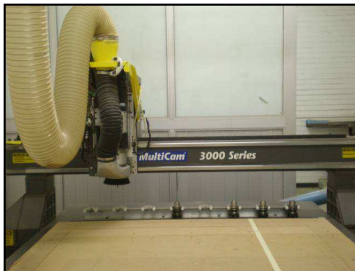
Figure 2: The Multicam ® CNC milling machine at DUT
