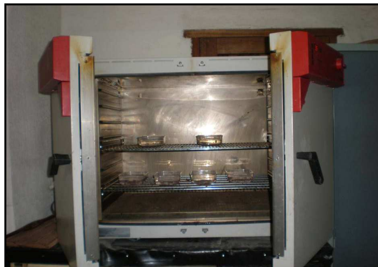
Figure 4: The Binder oven kept the specimens at a constant 37°C in distilled water
