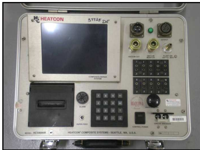
Figure 6: Heatcon ® 2000 hot bonding machine
