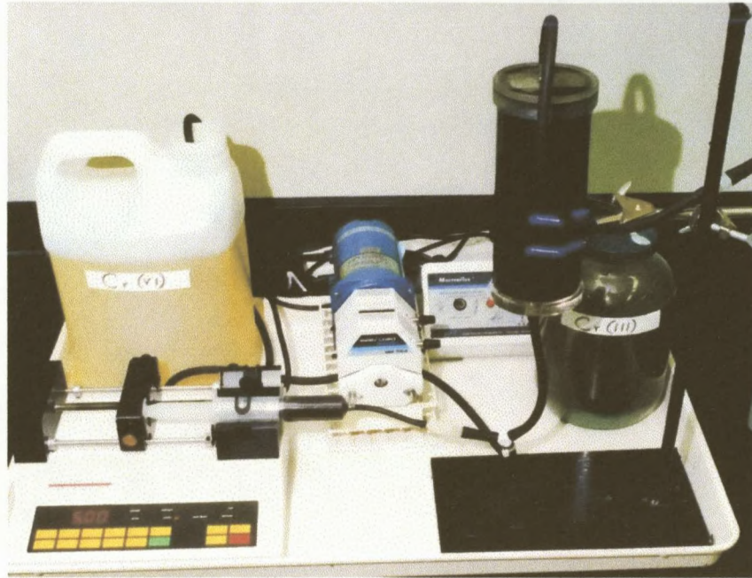
FIGURE 2.7 Bioreactor containing Cr(VI)-reducing bacteria for the reduction of Cr(VI) to Cr(III), Turick (1997).
