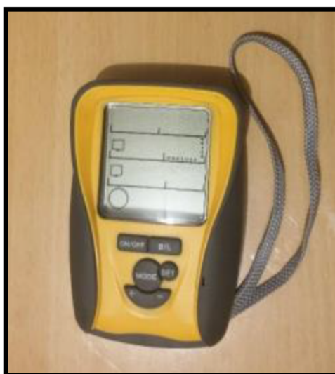
Figure 4-2: LCD digital pressure meter SCT-108.001.37
