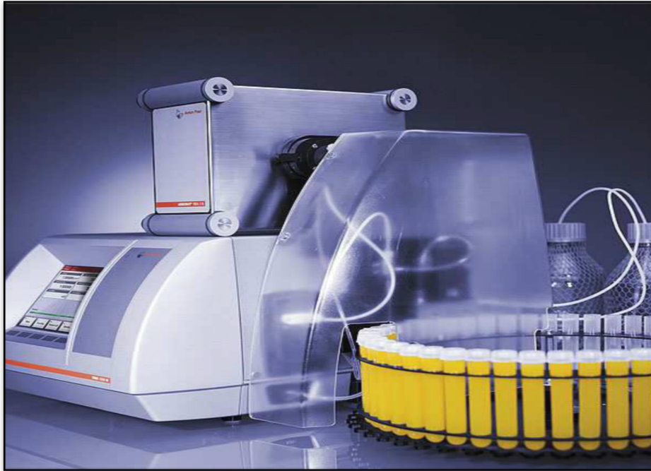
Figure 4.2: Photograph of the DSA 5000 M and the RXA 156 and Xsample 452 (Taken from Instruction Manual of Anton Paar DSA 5000 M)
