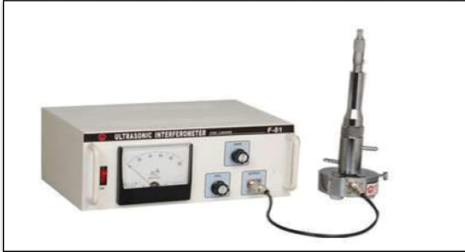
Figure 3.5: Photograph of an Ultrasonic Interferometer M-81G.
