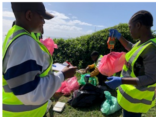
Figure 3.4: Fieldworkers weighing bin bags using a hanging scale and recording the weight
