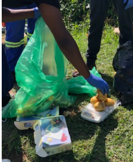
Figure 3. 5: Separation of food waste by food items and weighing using an electronic compact scale
