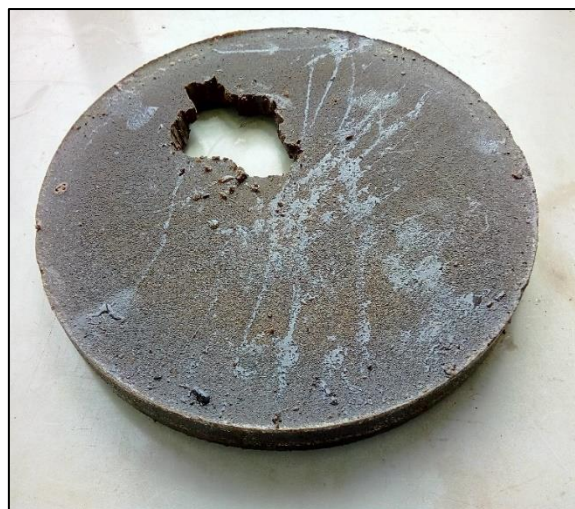
Figure 3- 3: Crude wax obtain via heating and melting method
