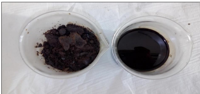
Figure 3- 4: Dried DAF mud (left) and molten crude wax (right)
