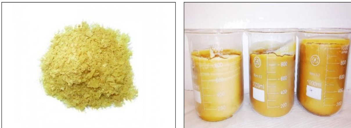
Figure 4- 19: Refined carnauba wax: literature (left) (ChemSrc, 2018) and of this study (right).
