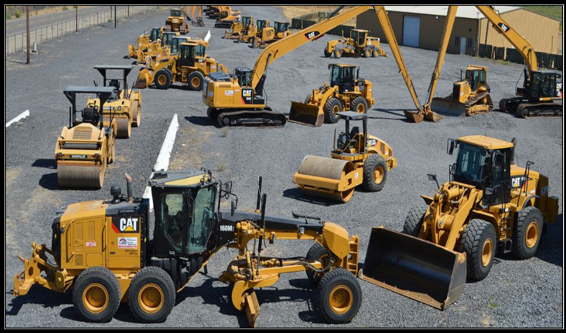
Figure 2. 5. Various types of plant machine used during TMM road formation construction (Anupoju, 2016)
