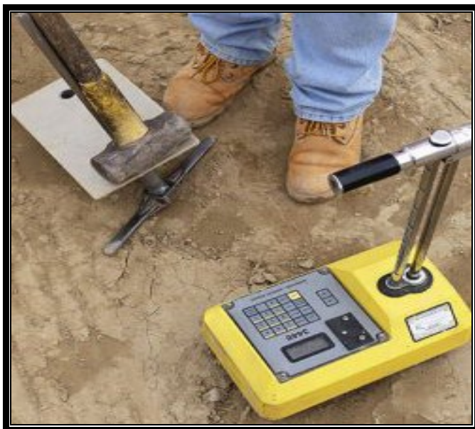
Figure 3. 6. Nuclear gauge or trolox used during density testing (Nuclear density gauge calibration, 2019)
