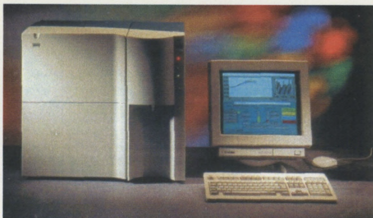
Figure 2.1 The AromaScanner A32/8S used in this study to analyze volatile compounds.
