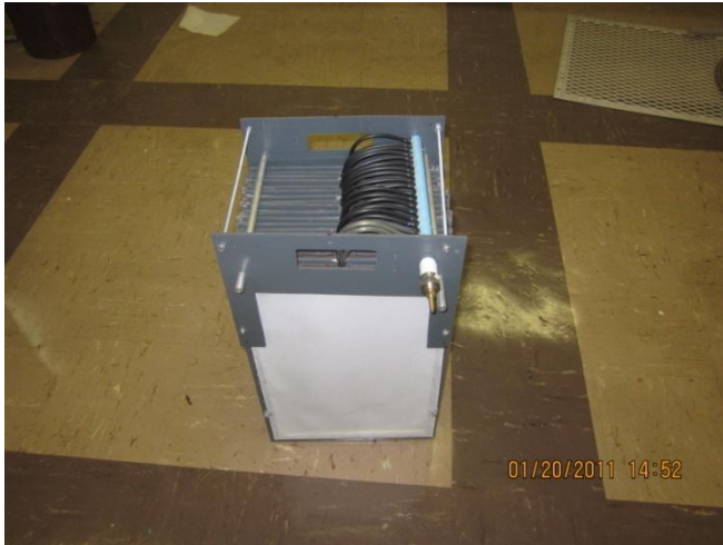
Figure 3.3: Membrane modules set up
