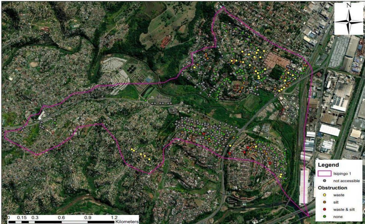
Figure 61: Isipingo 1 obstruction type.
