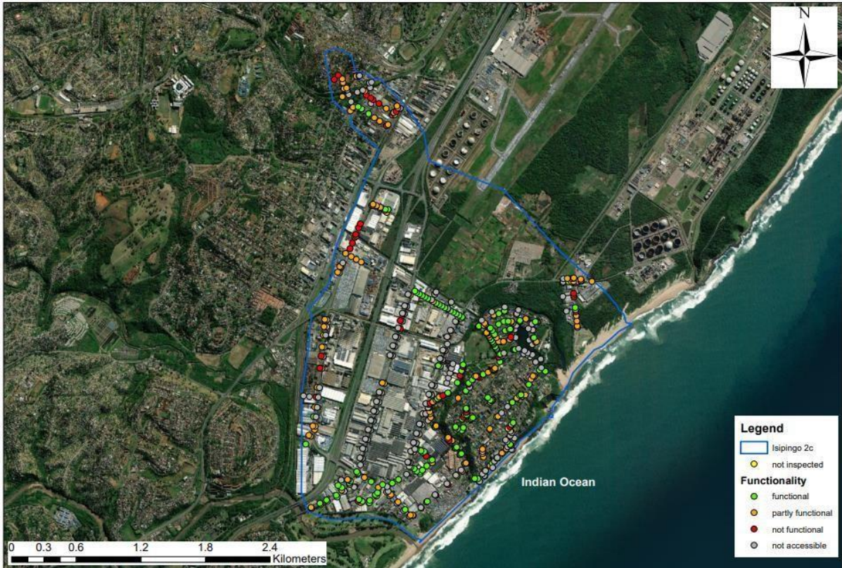
Figure 66: Isipingo 2c functional structures.
