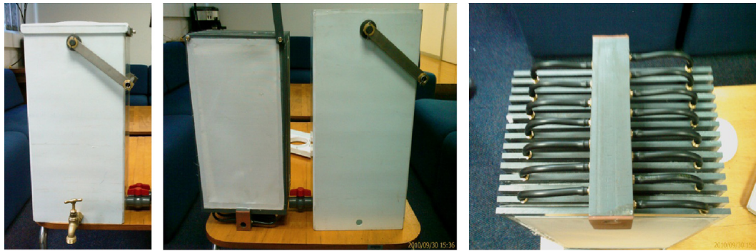
Fig. 1. The WFMFGF: assembled unit (left), front view (centre) and bottom view (right) of membrane pack.
