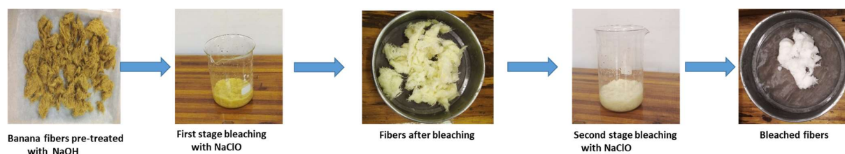
Figure 4. Two-stage bleaching process.
