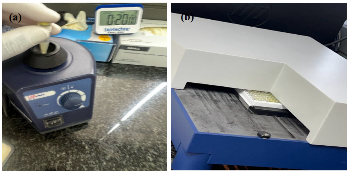
Figure 3.1: Instrument (a) Vortex and Timing devices; (b) Microplate reader.
