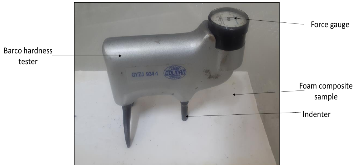
Figure 3.10: Figure 3.10: Barcol hardness test being conducted on hybrid filled foam composite core's surface
