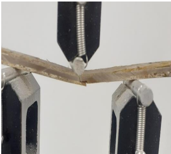
Figure 6.5: Flexural test set up showing sample after fracture
