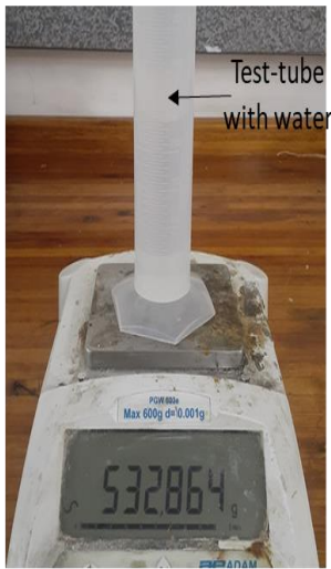
Figure 3.8: Buoyancy measurement procedure for HFFCs and SFCs
