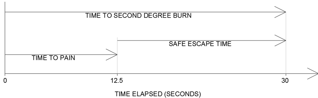
Figure 10: Safe escape time from 4.5 kW/m 2 heat flux exposure
