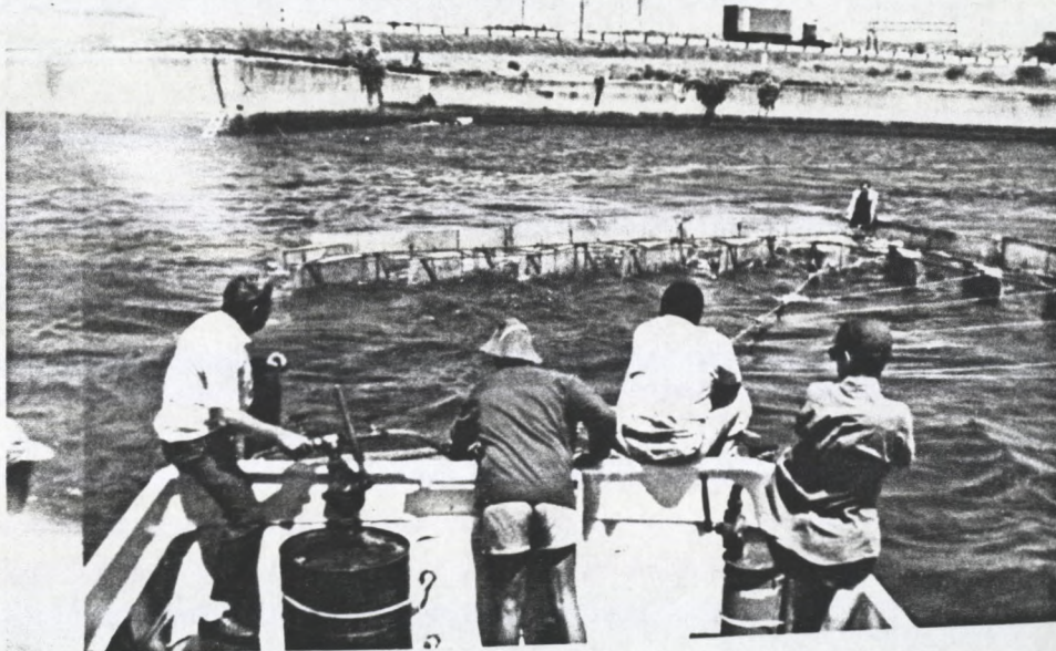
Figure 2.17. Oil being pumped from launch into bay ahead of prototype
