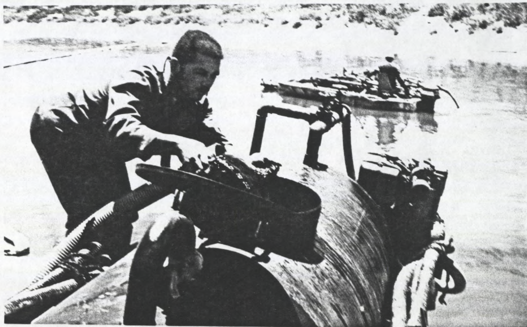
Figure 2.48. Pure oil being pumped from prototype into tank
