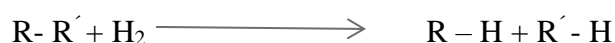
Scheme 2-9 Cracking reaction of long chain paraffins to smaller chain ones (Bezergianni, 2013b)
