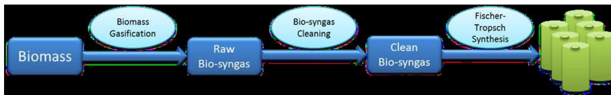
Figure: 2-9 Flow sheet of the Biomass to Liquid via Fischer–Tropsch Synthesis (BTL-FT) process (Freerks and Muzzell, 2004).
