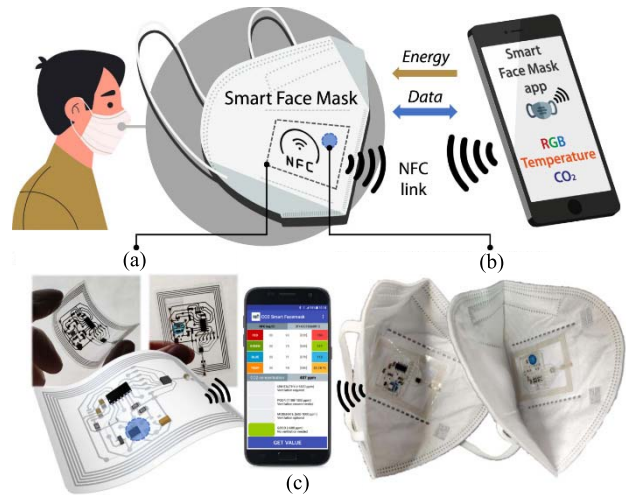
Fig. 3. Sample architecture of a SFM with CO 2 monitoring capability and its (a) NFC sensing tag, (b) CO 2 sensing layer, and (c) smartphone application for support [33].
