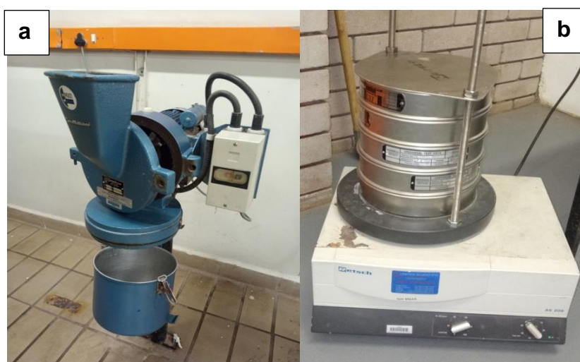
Figure 3.2: Images of (a) Attrition mill and (b) Mechanical sieve shaker
