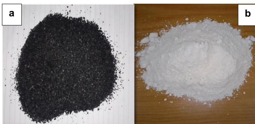
Figure 3.4: Images of adsorbents used in this study (a) Activated carbon (b) Kaolinite
