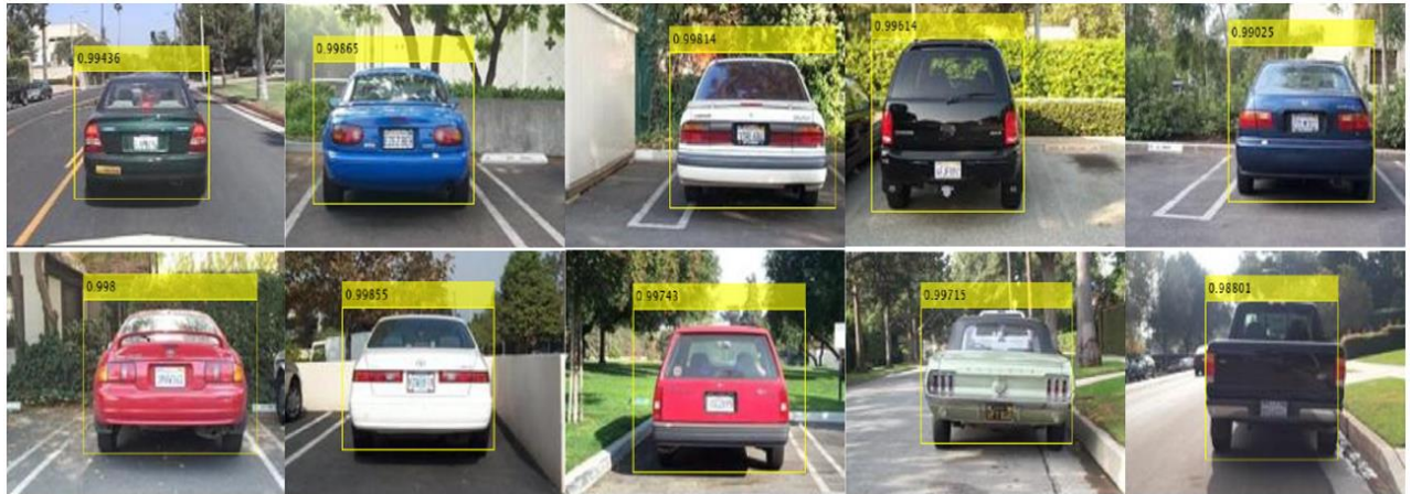
Fig. 4.10. Output results (mAP values) on a selection of test images for YOLO v3
