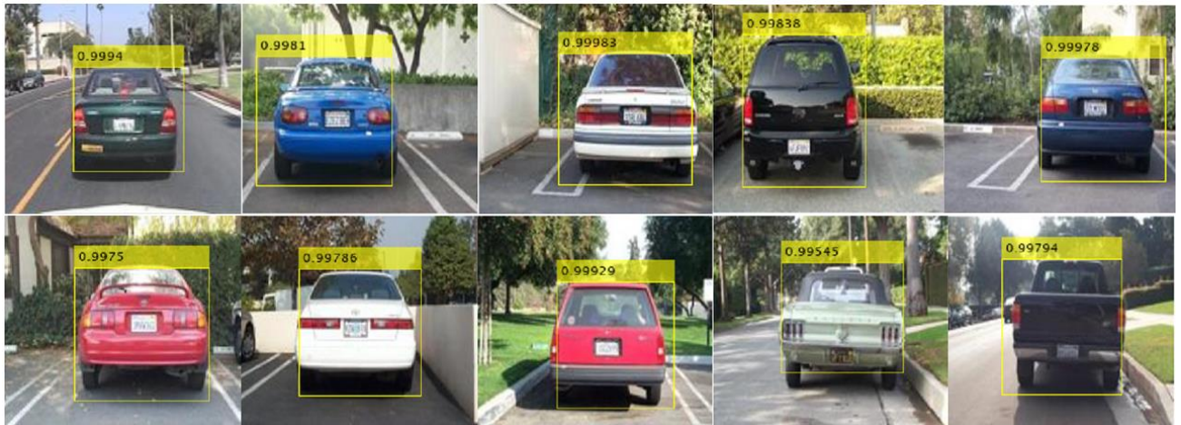
Fig. 4.5. Output results (mAP values) on a selection of test images for Faster R-CNN
