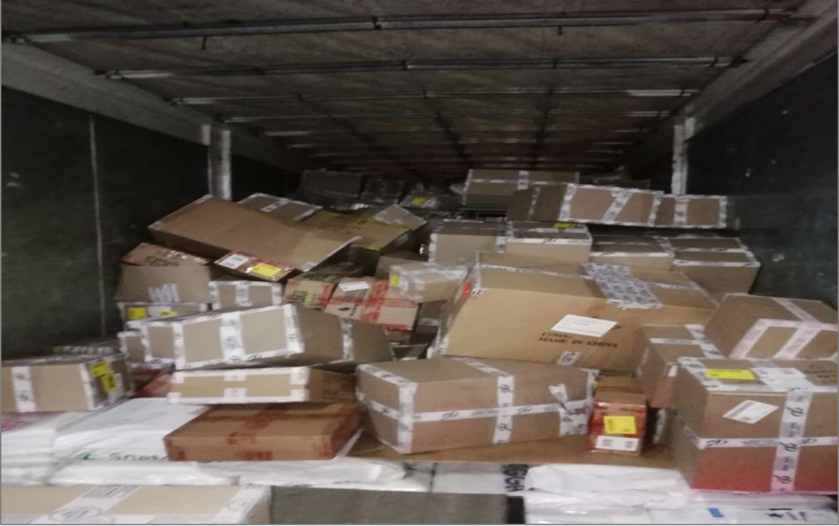
Figure 5.4: Illustration of poor load securement inside the distribution vehicle
