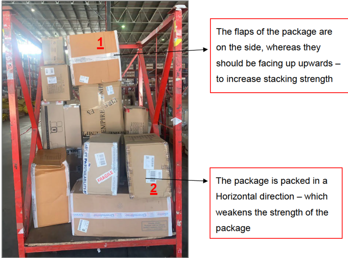
Figure 5.5: Illustration of poor methods of packing cardboard packages at storage
