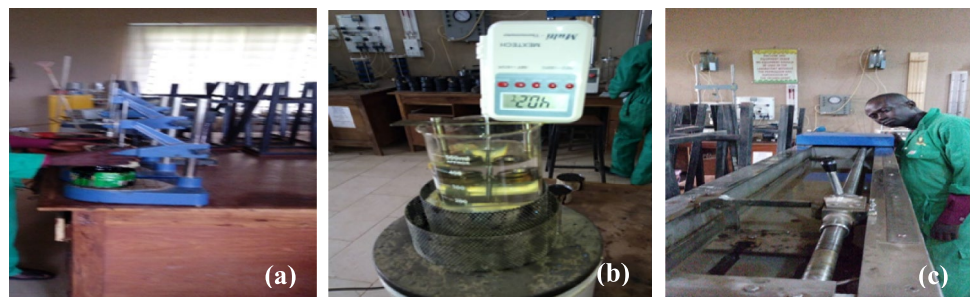
Fig. 2 Tests on asphalt binder a Penetration, b Softening point, and c Ductility
