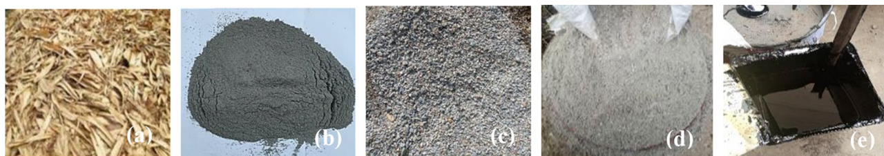
Fig. 1 Materials used a Dry Bambusa vulgaris leaf, b Bambusa vulgaris leaf ash, c Coarse aggregate, d Fine aggregate, and e Asphalt binder
