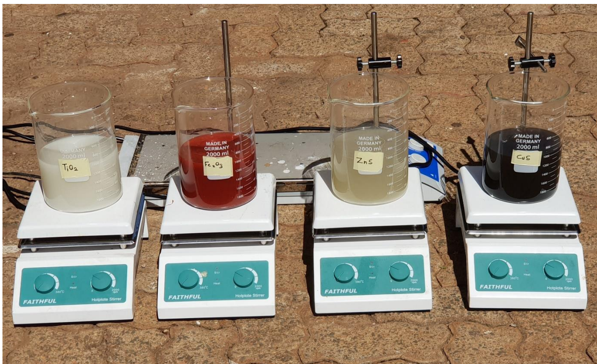
Figure 3-3: Demonstration of the photocatalytic degradation wastewater treatment system experimental set-up using sunlight irradiation
