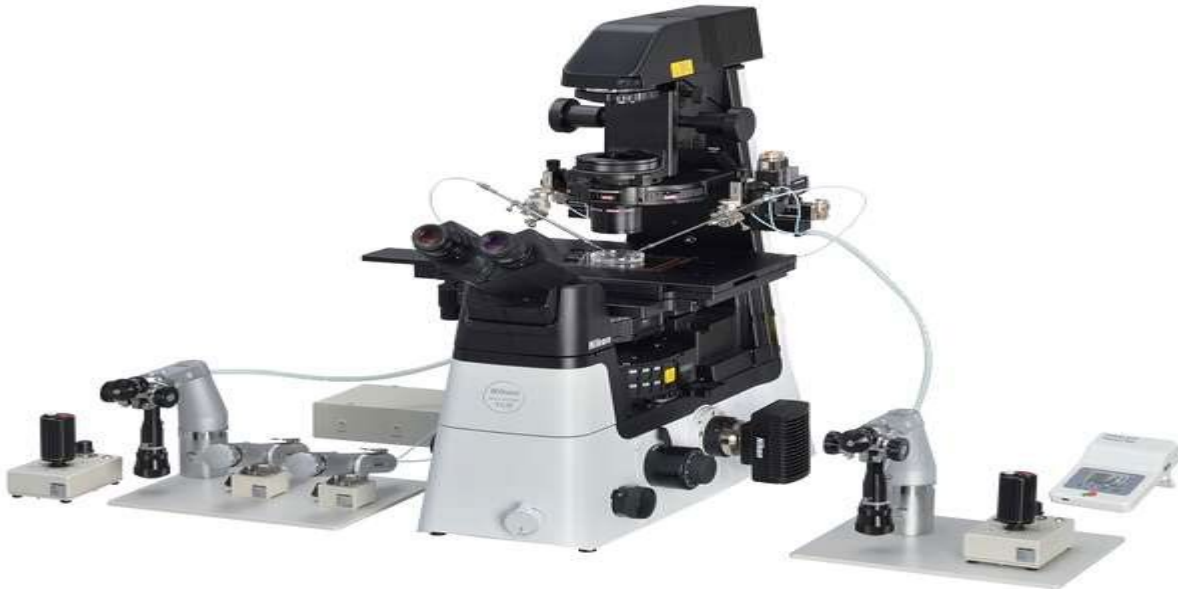
Fig. 2.4: Illustration of micromanipulator used for cell isolation
