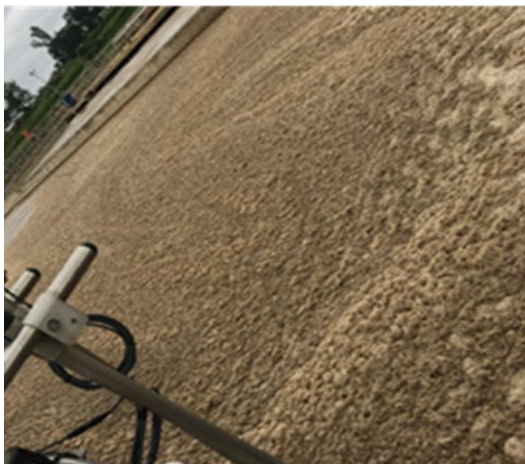
Fig. 4.1: Foaming sludge observed from WWTW B during sampling. This sampling episode was observed in June.
