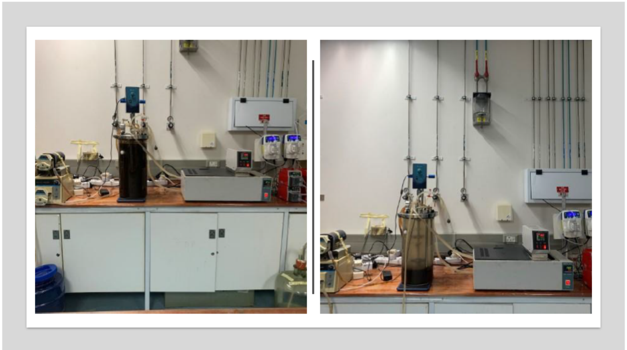
Plate 1. Photographic image of Anammox enrichment reactor.
