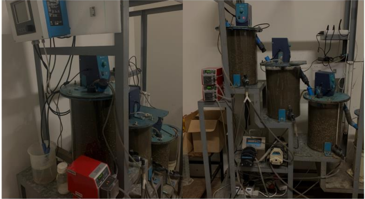
Plate 11: Photographic image of SPDA Reactor treating real municipal wastewater
