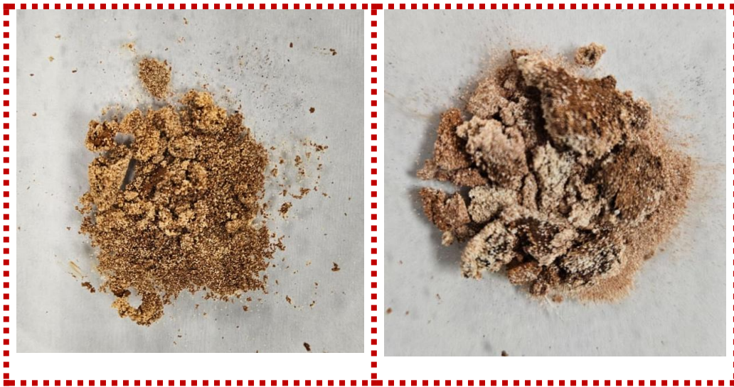
Figure 43: Images of used (a) g-C 3 N 4 @Fe 3 O 4 , (b) BNNS@Fe 3 O 4 showing the adsorption of MPs onto the MNCs after treatment
